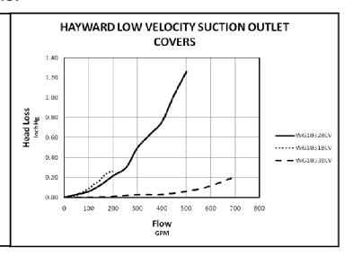
WG1031BLV Suction Outlet Cover (Replacement sold as a WGX1031BLV) is rated for 108 GPM Wall Mounted or 190 GPM Floor Mounted for single or multiple suction outlet use. (9" x 9")
